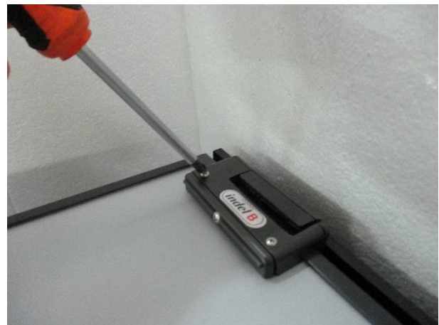
4. Remove the handle (3 screws)
