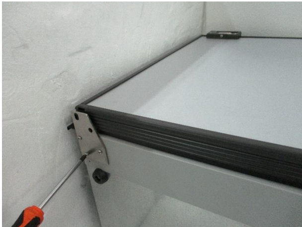
1. Unscrew the 2 hinges (6 screws)
