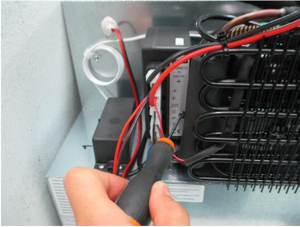
1. Unscrew the bolt fixing the ECU
