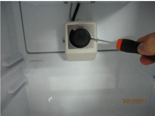
3. Use a screwdriver as a leverage to remove the thermostat's knob
