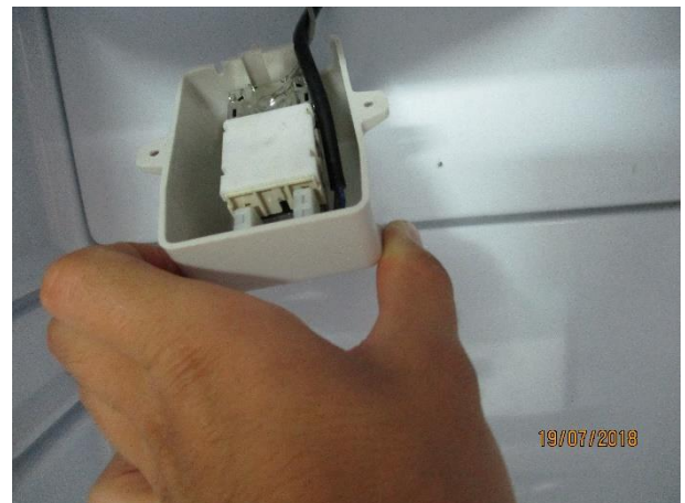
6. Pull the thermostat to remove it and reverse the procedure to replace it
