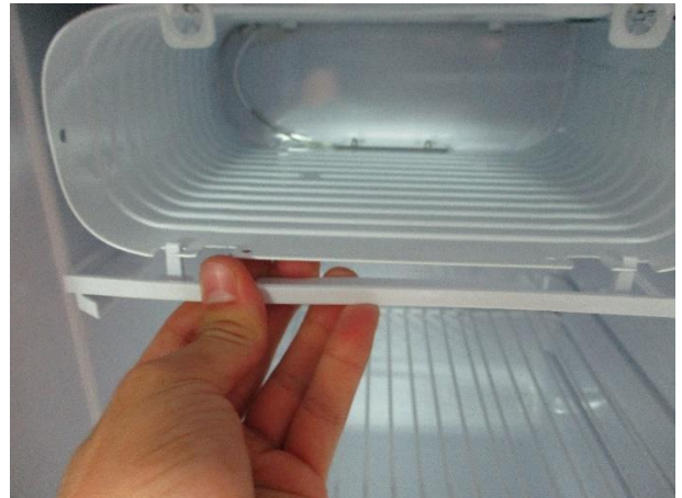
2. Remove the plastic protection
