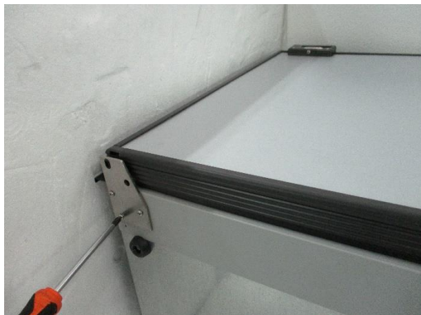
1. Unscrew the 2 hinges (6 screws)
