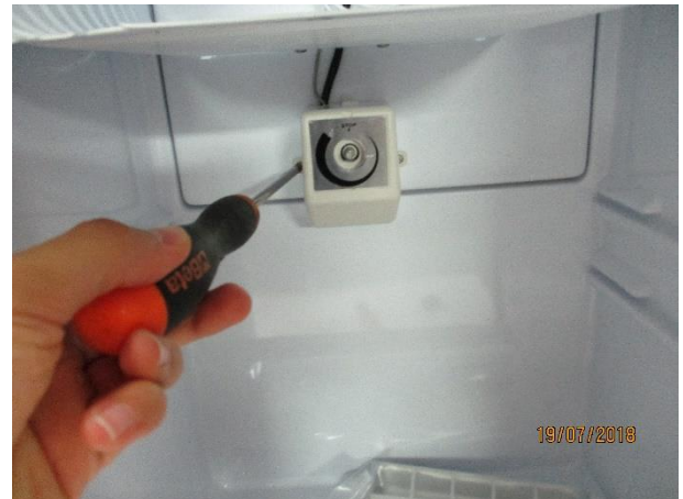
4. Unscrew the 2 bolts fixing the thermostat
