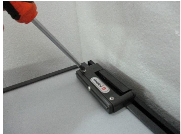
2. Unscrew the handle (3 screws)
