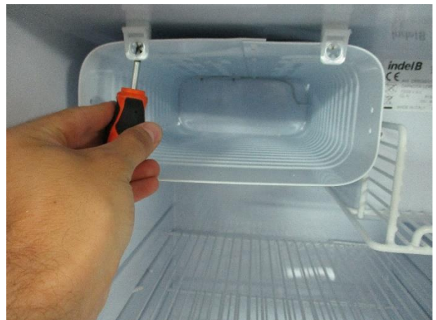
4. Unscrew the 2 bolts fixing the freezer
