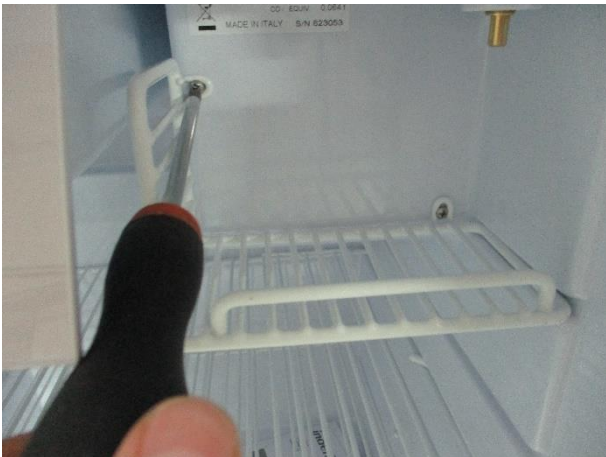
7. Unscrew the grid (2 screws)
