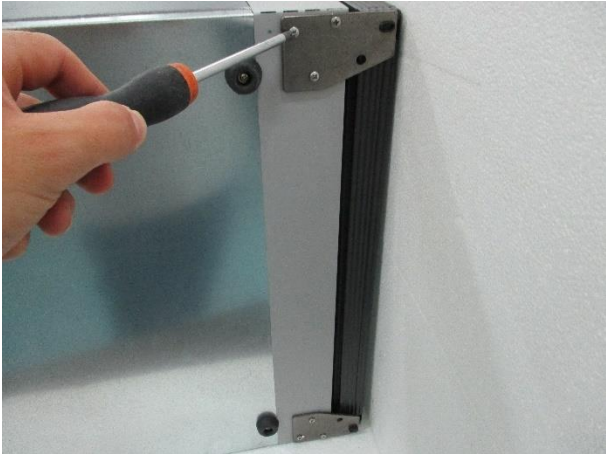
1. Unscrew the 2 hinges (6 bolts)
