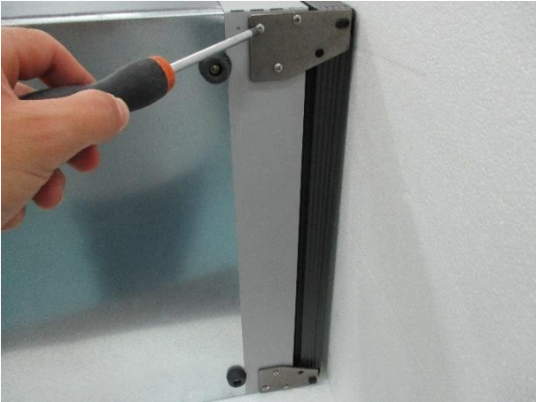
1. Unscrew the 2 hinges (6 bolts)
