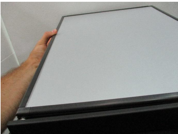
3. Lift the door from the opposite side of the screw nut to remove it. Reverse the procedure to replace it
