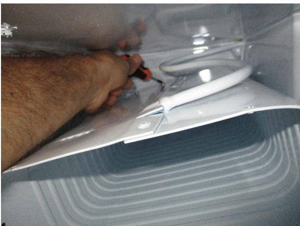
5. Unscrew the 2 bolts fixing the thermostat
