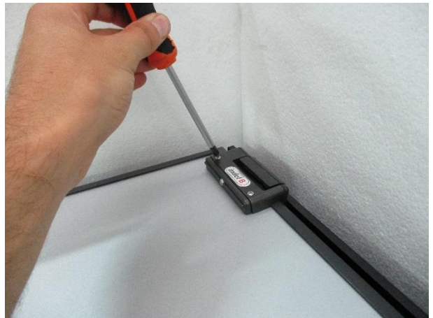
4. Unscrew the handle (3 bolts)
