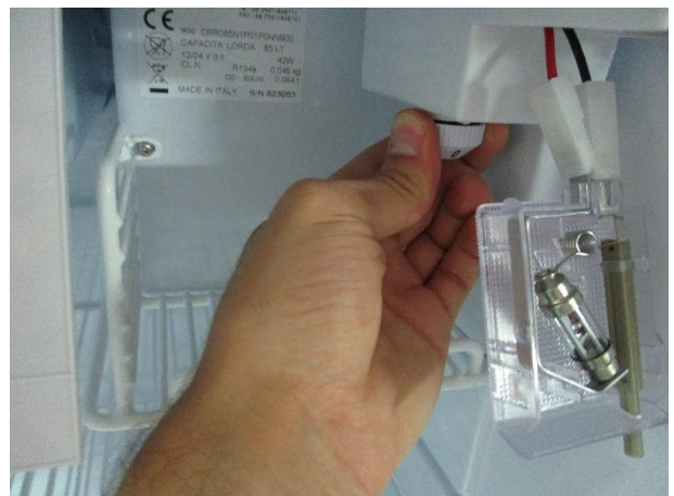
6. Unscrew the light bulb and remove the thermostat knob
