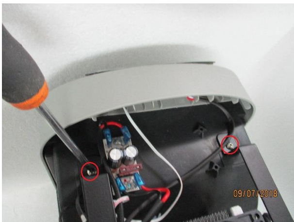
5. Unscrew the 2 bolts fixing the 2 brackets
