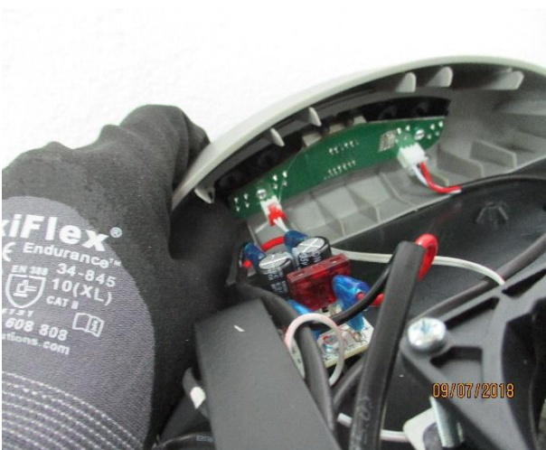
4. Press on the interlock to remove the display
