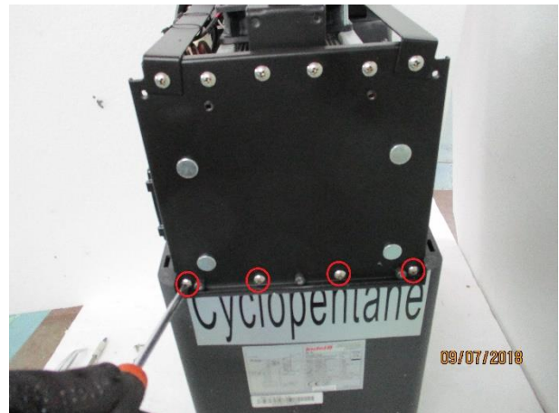
4. Unscrew the 4 bolts highlighted in figure
