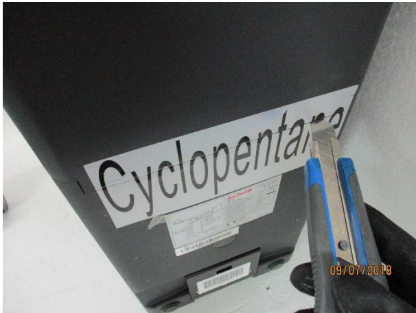
1. Cut the label and remove it
