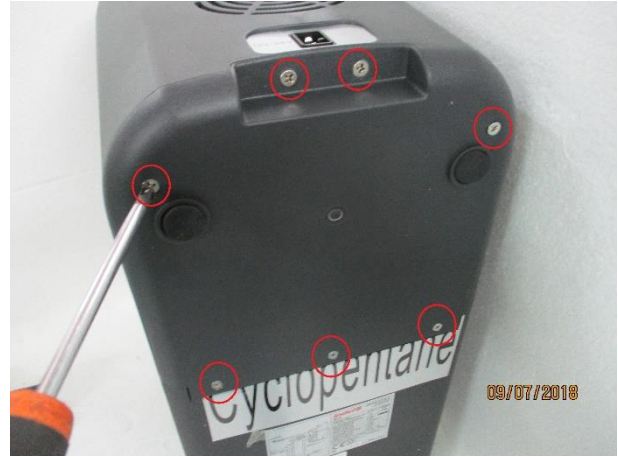
2. Unscrew the bolts fixing the cover (7 bolts)
