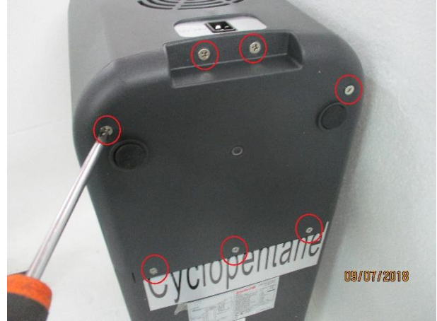
2. Unscrew the bolts fixing the cover (7 bolts)
