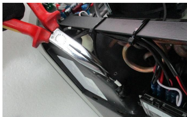
5. Disconnect the wire that connect the temperature sensor and the ECU, remove the sensor and reverse the procedure to replace it
