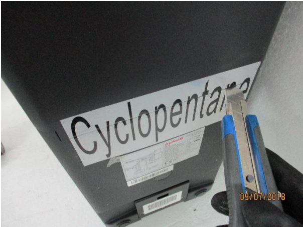
1. Cut the label and remove it
