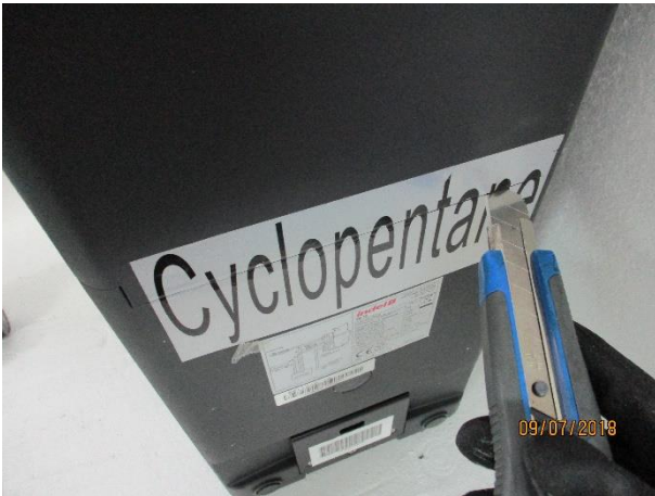
1. Cut the label and remove it
