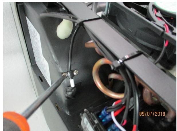
4. Unscrew the 2 bolts fixing the sensor
